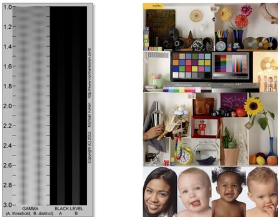
Figure 3. Monitor calibration images: on the left, Norman Koren's monitor gamma chart, and on the right, the Photodisc color calibration image. These printed examples should not be used for reference as their colors may have changed due to printing press inconsistencies.
